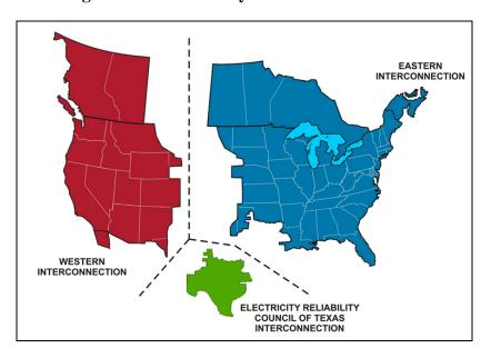
Figure 1. U.S. Power-System Interconnections<sup>4</sup>
